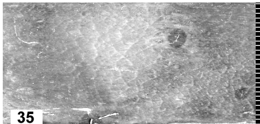
Fig.4 Typical Soot Track Record of the Re-initiation from a Multiple Holed Plate
